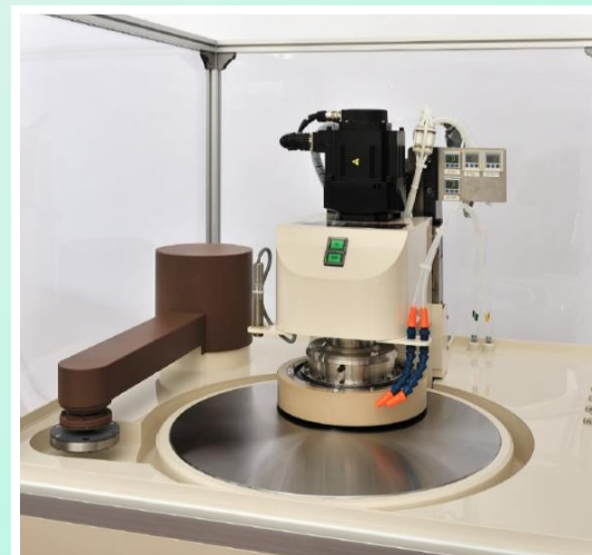
Conditioner at "home" position
